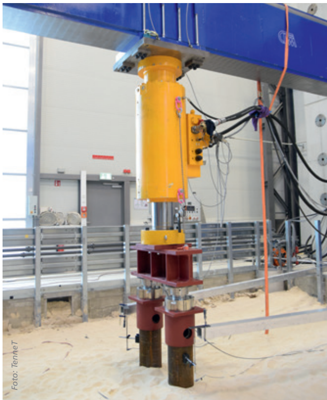
Investigating the impact on the load bearing capacity of piles arranged as a dyad
