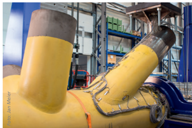
Welded nodes of a jacket structure prepared for testing
