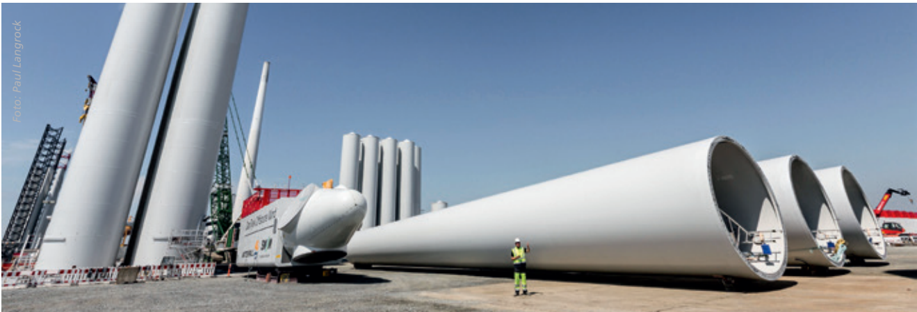
Monopiles and tower segments arranged for removal
