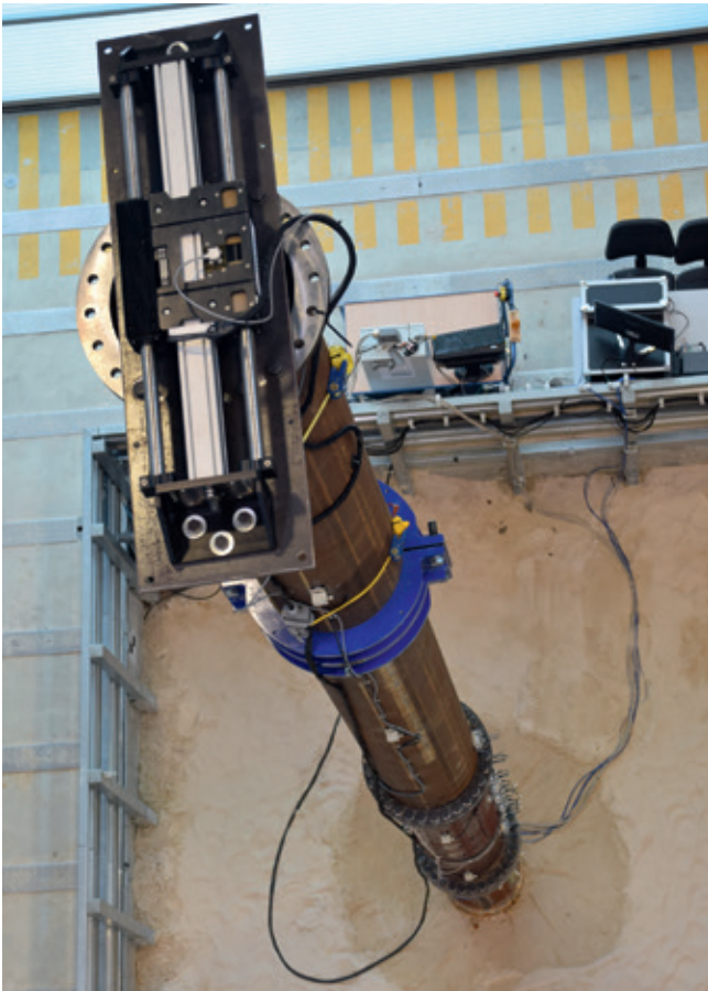
Investigation of the structural dynamic behavior of monopiles
